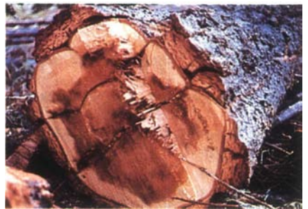
Figure 32. — Cross section at the base of a white fir showing frost cracks, shake, and wetwood.
