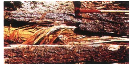
Figure 9. — Felled white fir that split, showing stringy nature of decay from rust-red stringy rot.
