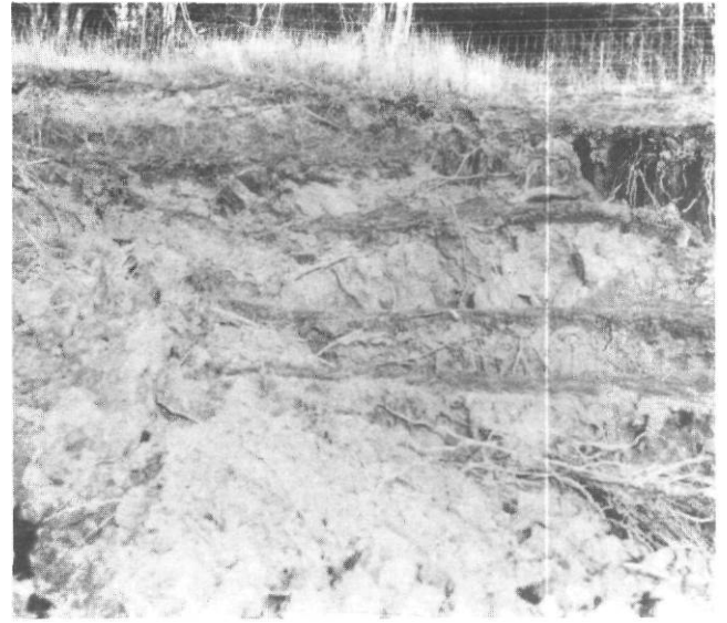
Figure 14.--Hummocky surfaces (upper left). An irregular, hummocky surface shows that the soil mantle has been undergoing forces which cause deformity and movement. These are risky locations for roads without proper investigations and design for the situation.
