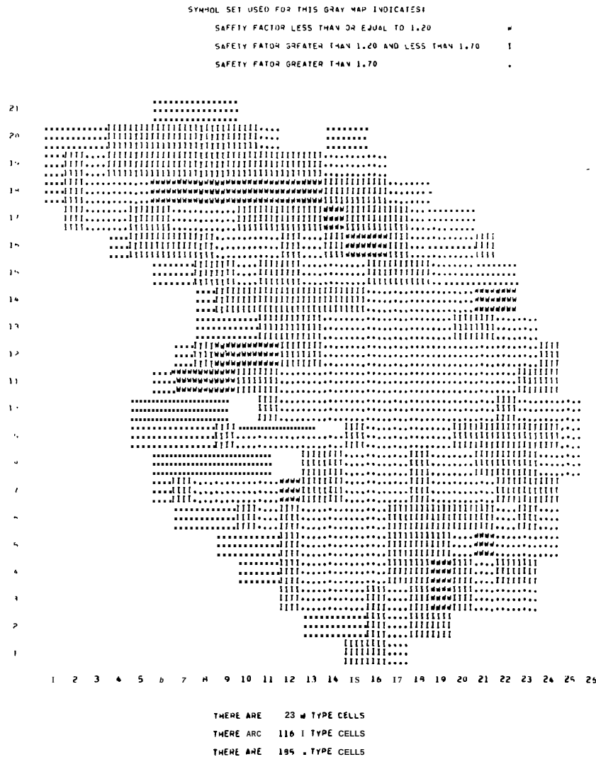
Figure 3.—Gray area or print density map of Starfish Creek, Alaska, showing changes in factors-of-safety resulting from 100 percent reduction in timber density (entire area clearcut).
