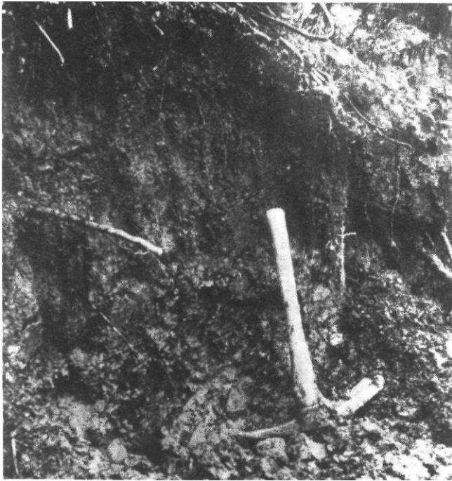
Figure 5.--Gleyed or mottled soil. A gleyed soil exhibits gray or bluish colors because iron is reduced chemically. A high water table usually occurs continuously or for long periods of time annually in gleyed soils.
