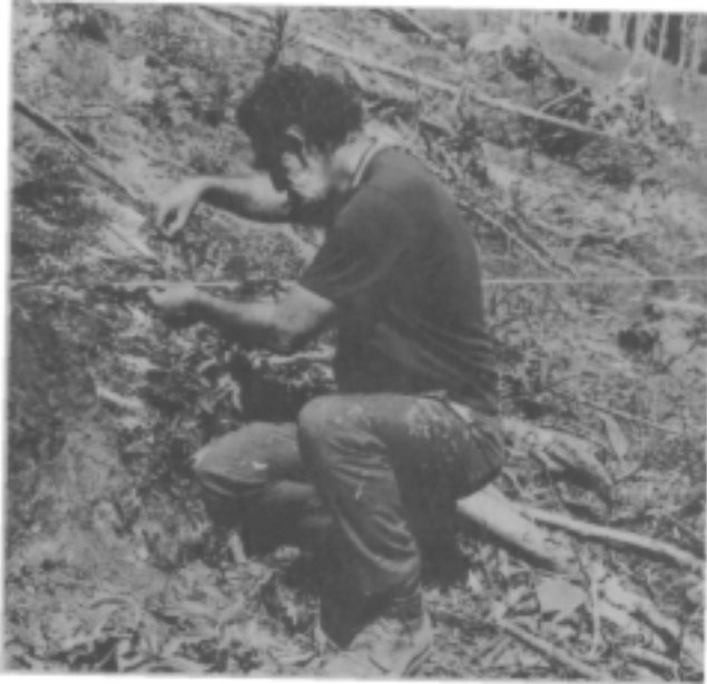
Figure 3.--Measuring vertical displacement of soil.
