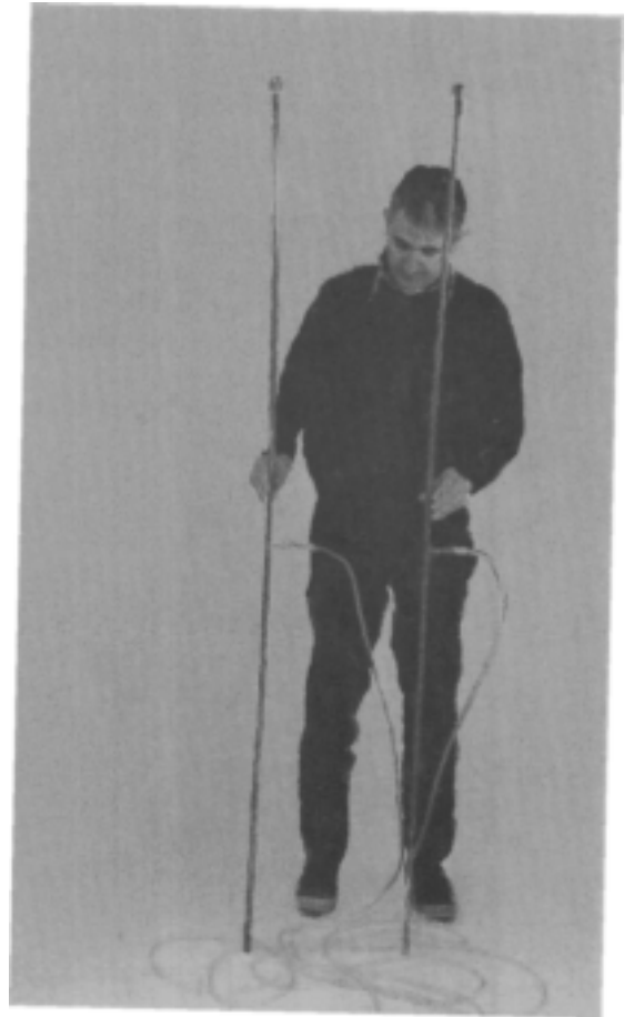
Figure 1.--The waterlevel device.
