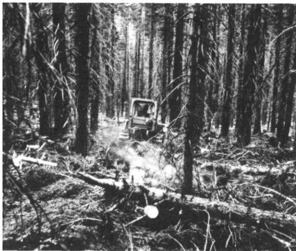
Figure 11.—Using small skidders reduces injury to residual trees in young stands. Equipment suitable for old-growth stands is not suitable for young-growth stands, although it is often used for thinning.
