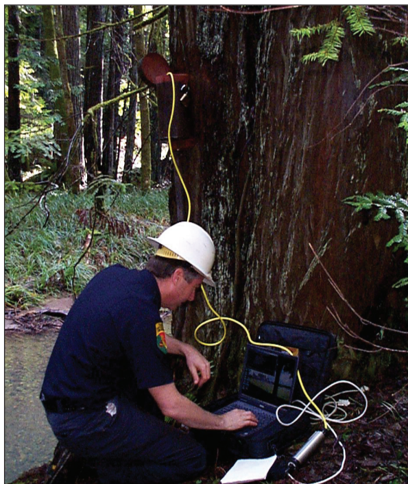
Collecting stream flow data at Jackson Demonstration State Forest. The data logger takes a sample every 30 minutes.
