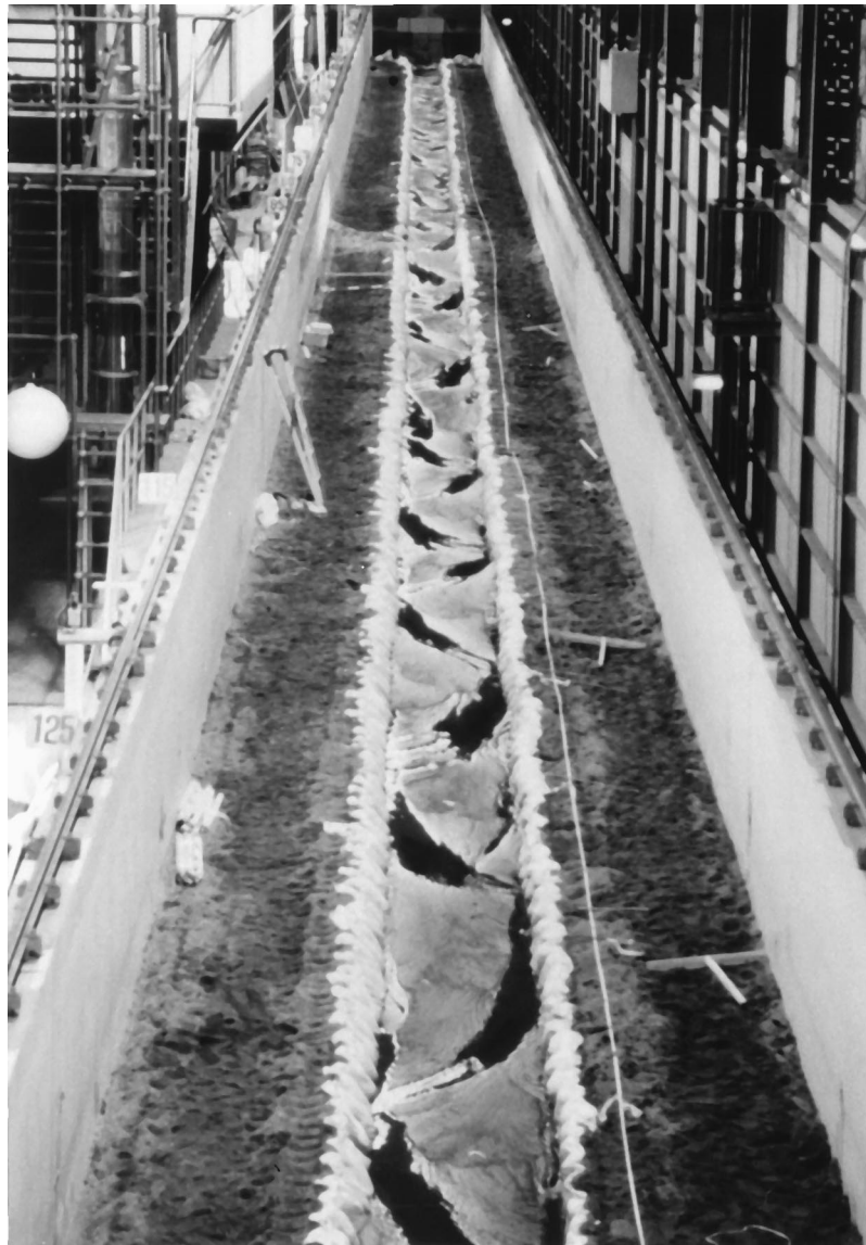
Figure 1. The Large Flume, Environmental Research Center, Tsukuba University, looking upstream after the sediment wave was introduced. The flume has been mostly drained to reveal alternate bars. The regularity of the bars in the far foreground has been disturbed by the wave.
