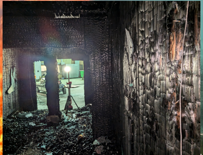
A look inside one of the compartments following the fire test. Forest Service photo by Laura Hasburgh.
