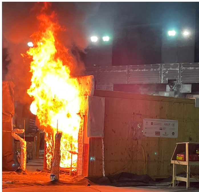
Fire testing underway in one of the WOODWISE compartments. Forest Service photo by Kara Yedinak.
