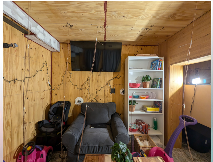
Modern fuels inside one of the WOODWISE compartments. Researchers used a variety of household objects made from assorted materials. Forest Service photo by Kara Yedinak.
