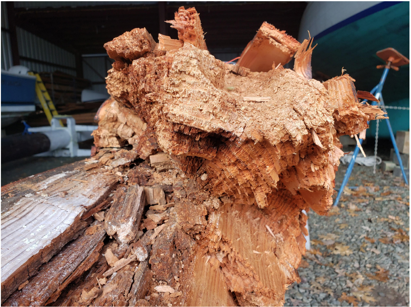
Figure 1F. —Close up of fractured cross section of the Grace Bailey mast. Forest Service photo by Xiping Wang.
