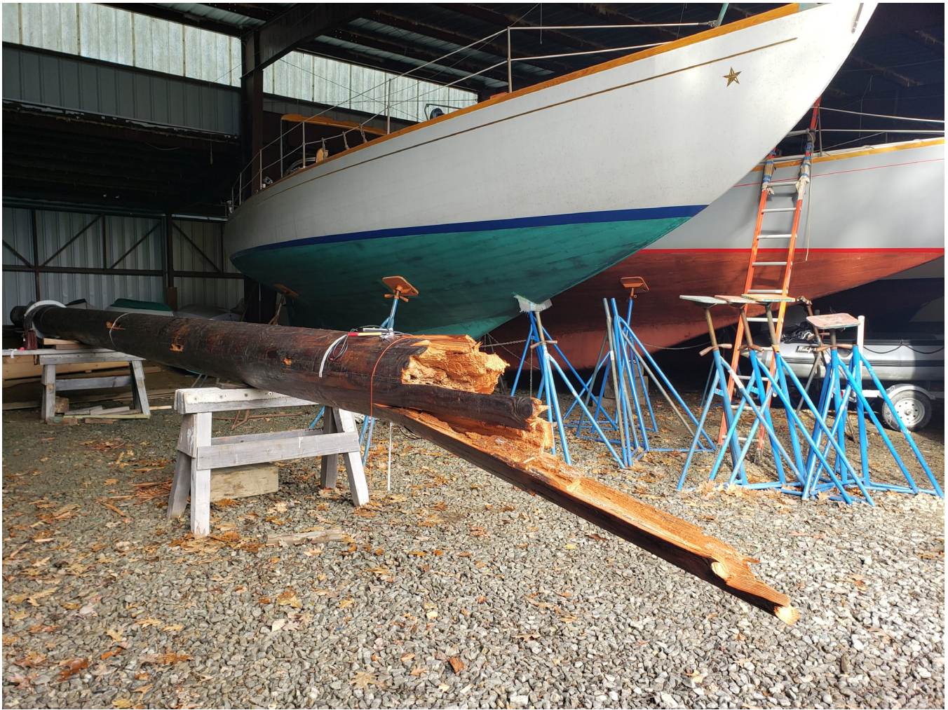
Figure 1C. —Fracture of the Grace Bailey mast (lower portion). Forest Service photo by Xiping Wang.
