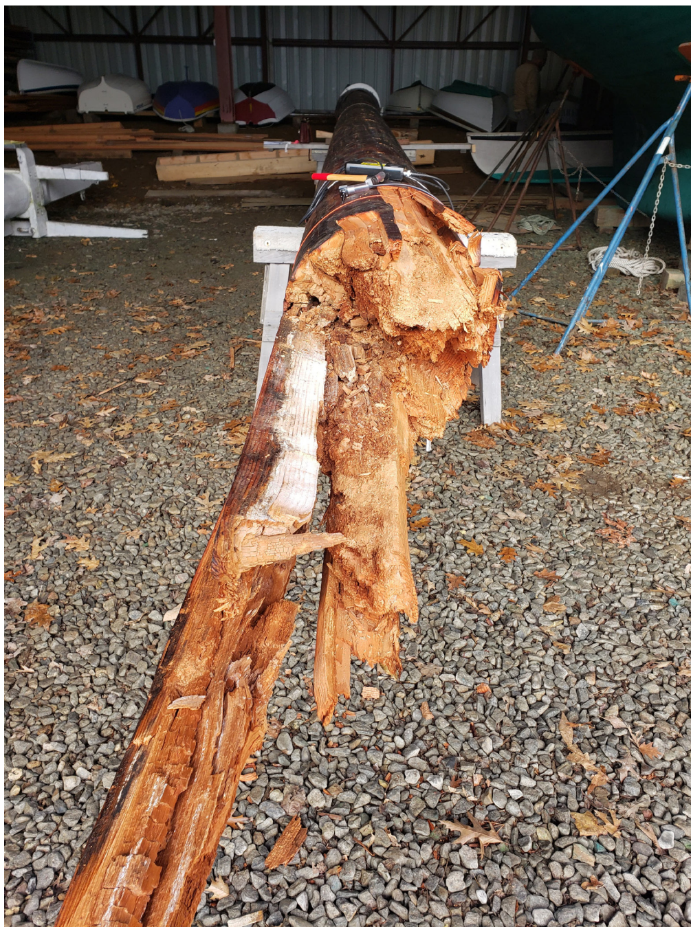
Figure 1D. —Fracture surface of the Grace Bailey mast (upper portion). Forest Service photo by Xiping Wang.
