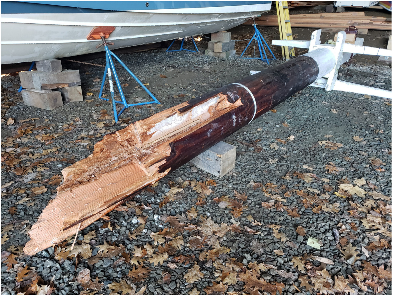
Figure 1B. —Fracture surface of the Grace Bailey mast (upper portion). Forest Service photo by Xiping Wang.
