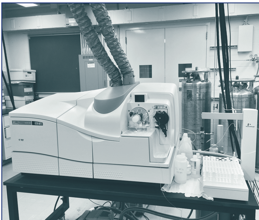
Figure 15. The scientists used a Perkins-Elmer ELAN 6000 ICP-MS to analyze the sediment samples. This equipment enabled the scientists to identify a wide variety of chemical concentrations in the sediment samples. Photo courtesy of Dr. Daniel Bain and the University of Pittsburgh.
