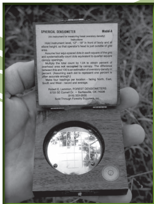
Figure 8. A densiometer measured the amount of canopy cover. Canopy cover is the percentage of leaves shading the ground. Photo courtesy of University of Georgia Warnell School of Forestry and Natural Resources. Photo by Jean Szymanski.
