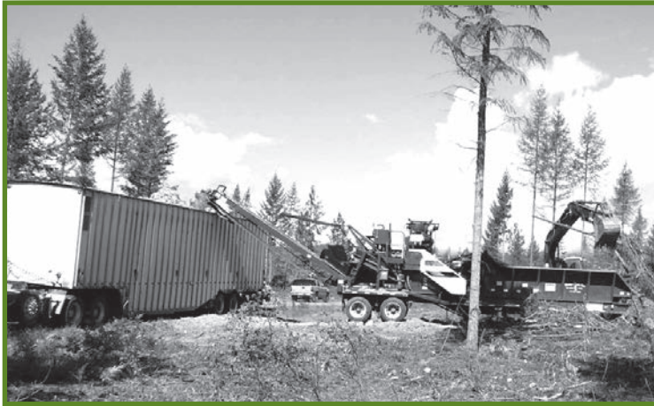
Figure 8. Large chipping machines turn large trees into small chips of wood. Photo courtesy of the U.S. Forest Service.
