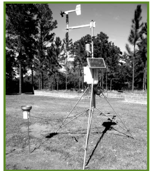
Figure 7. Weather stations were set up to measure air temperature, relative humidity, wind speed, and rainfall. This is a weather station at the University of Georgia. Photo courtesy of University of Georgia Department of Geography. Photo by Jean Szymanski.
