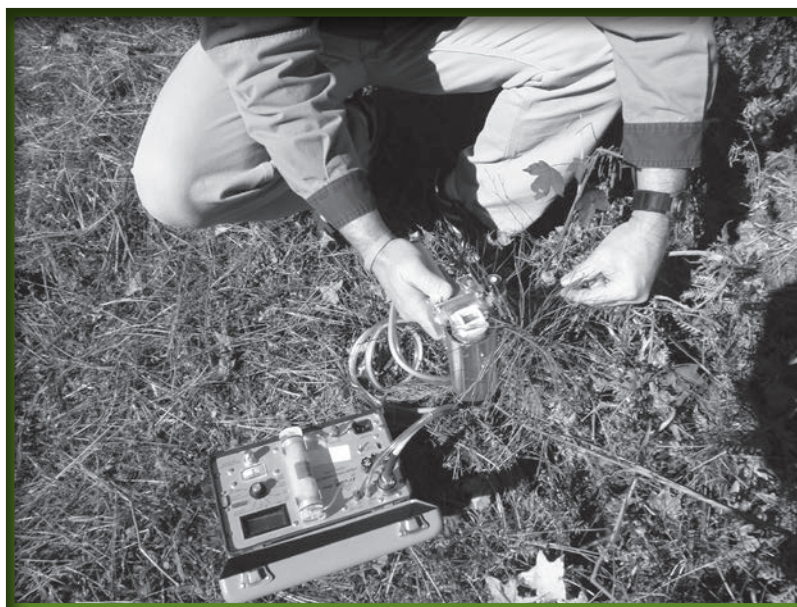
Figure 9. A porometer measured the amount of CO 2 entering and the amount of water exiting a leaf pore. Photo courtesy of University of Georgia Warnell School of Forestry and Natural Resources. Photo by Jean Szymanski.
