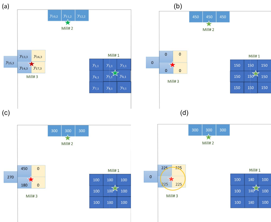
Fig. 1 (a) Hypothetical county draw map of a 3-mill stratum ( k is omitted here), ( S_k = \{1, 2\} ); y_{ij} is the sawlog volume sourced from county i for mill j . Stars indicate the locations of the three mills, while rectangles represent individual counties in a state. (b) Sawlog volume estimates \hat{y}_{ij} from TPO method. (c) Sawlog volume estimates \hat{y}_{ij} from HP method. (d) Sawlog volume estimates \hat{y}_{ij} from RP method. The circle illustrates a 25-mile sourcing radius from the mill
