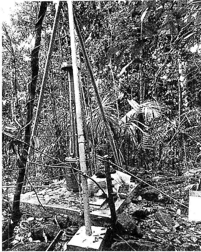
Fig. 5.4 The radiation source used to irradiate the wet forest at the El Verde sector of the Luquillo Experimental Forest. The two-ton lead container at the center of the concrete base contains the radioactive Cesium source, which when in operation, would be magnetically hoisted to below the oval metal structure at the top of the aluminum shaft. (From Odum 1970c)
