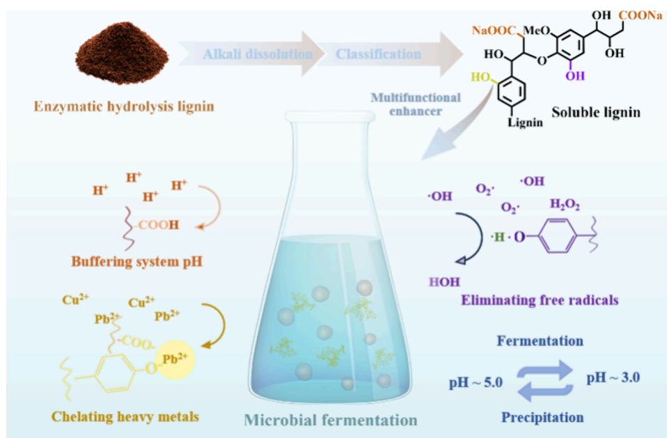
Figure 1. Schematic diagram of soluble lignin as a microbial fermentation enhancer.
