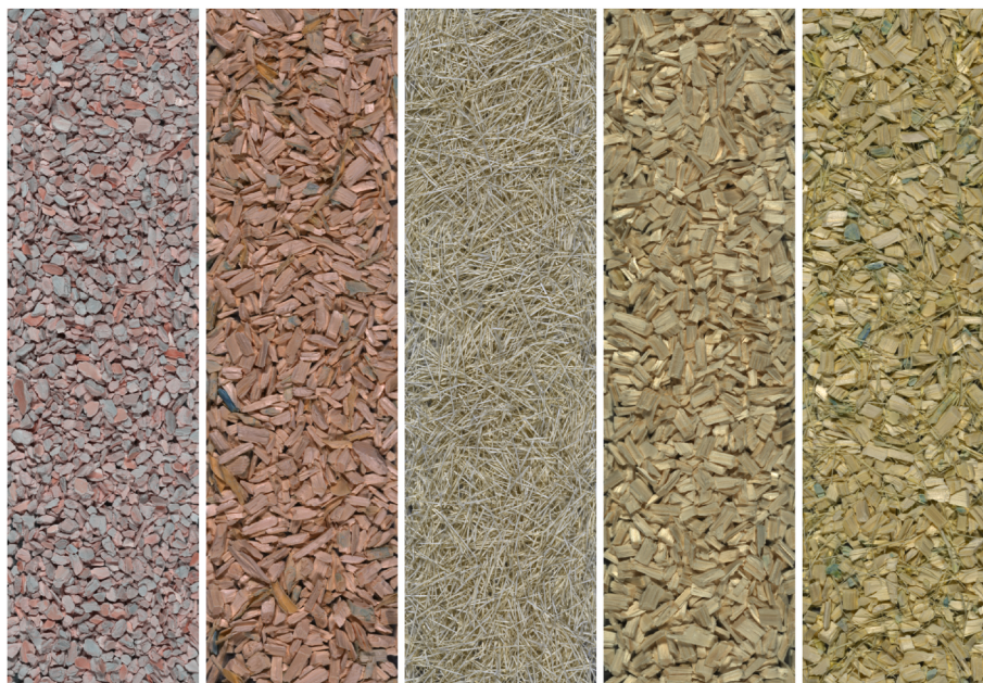
Fig. 2. Pseudo-color images from the hyperspectral imaging setup for bark, branches, needles, wood, and the mixed fraction from the 7 mm size class. (For interpretation of the references to color, refer to manuscript text where this figure is referenced.)
