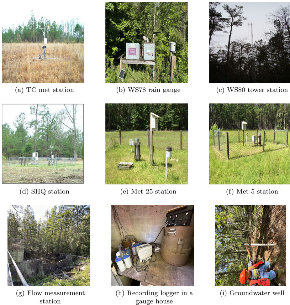
Figure 3. Photos of various hydro-meteorologic measuring equipment on the study watersheds. Met 5 and Met 25 are satellite stations measuring air temperature, soil temperature, and precipitation on WS77 and WS80, respectively. TC met is the complete weather station on the WS78 watershed. SHQ is another full-weather station in the headquarters office.
