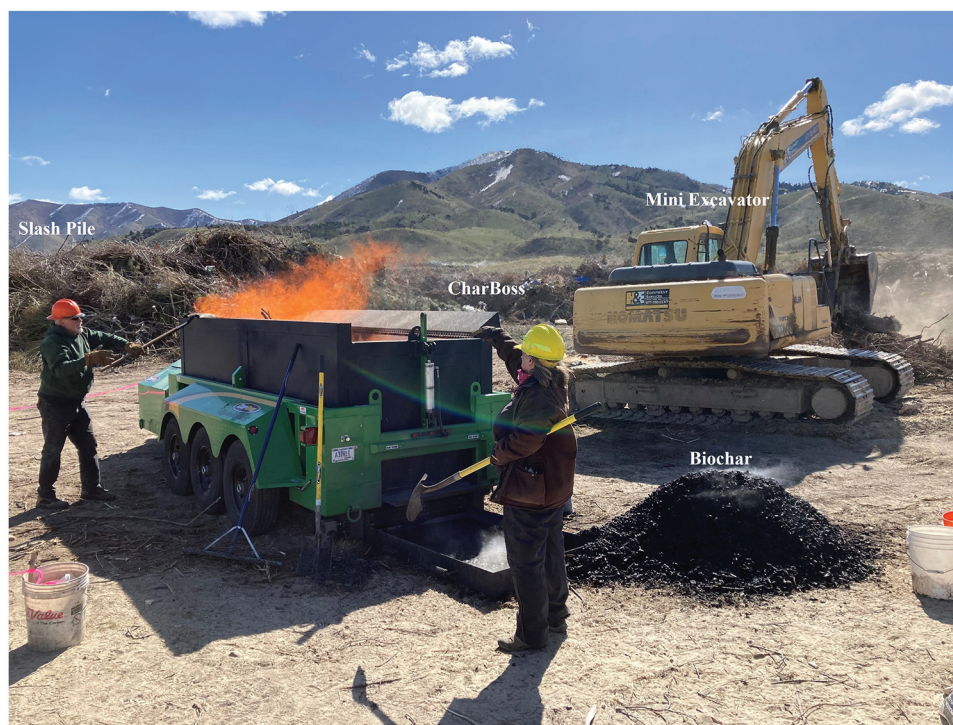
Figure 1. CharBoss operations producing biochar. Photo: U.S. Forest Service.
