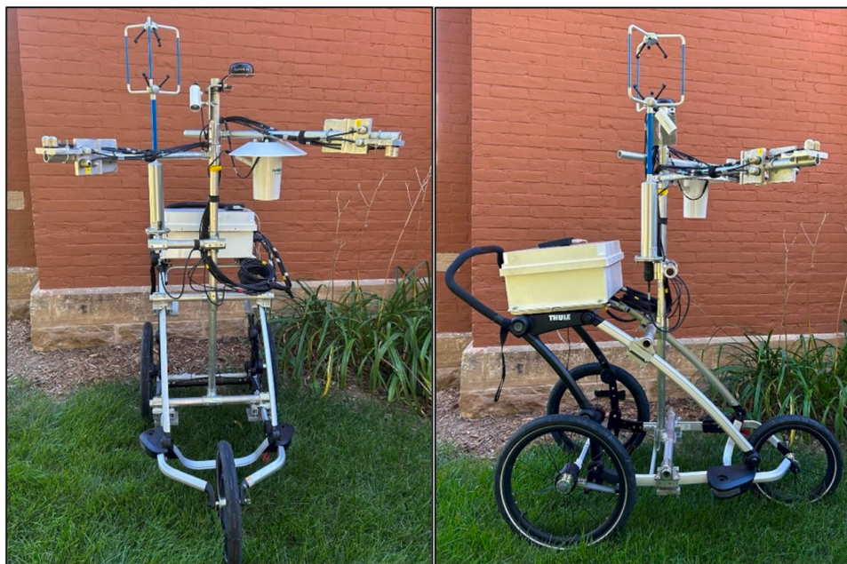
Fig. 3. The MaRTa machine, equipped with shortwave and longwave radiation sensors in six directions, along with sensors for other metrics including air temperature, relative humidity, and wind velocity.
