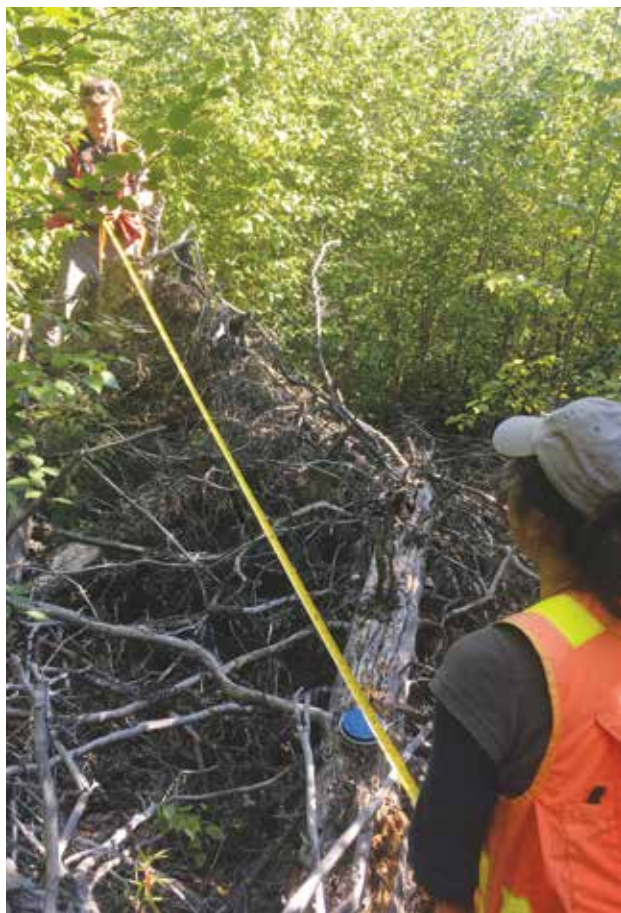
Figure 28—State of Alaska crew members measure down woody material on a Forest Service, Forest Inventory and Analysis (FIA) plot. Measured down woody material includes coarse woody debris ( \geq 3 inches diameter) and fine woody debris ( < 3 inches diameter) intersected by eight 24-foot transects per FIA plot. Photo courtesy of Joe Vorderbruggen, State of Alaska.
