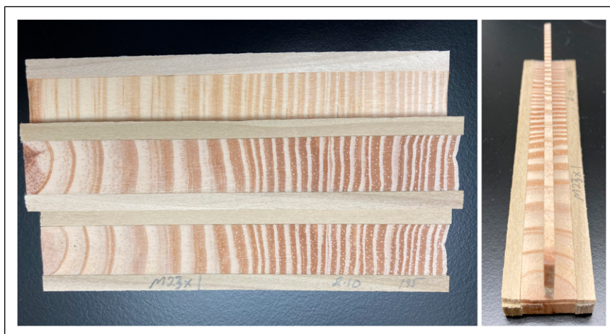
Figure 1. Left image shows the acetone-soluble extractives sample (2.5-mm transverse thickness), ultrasonic velocity sample (8.5-mm longitudinal thickness), and the X-ray sample (2-mm longitudinal thickness); right image shows the same samples, but the transverse view of the acetone extractives sample. Note the aligned growth rings for the samples and the yellow poplar strips on the edges of the samples which were removed prior to determining extractives content.
