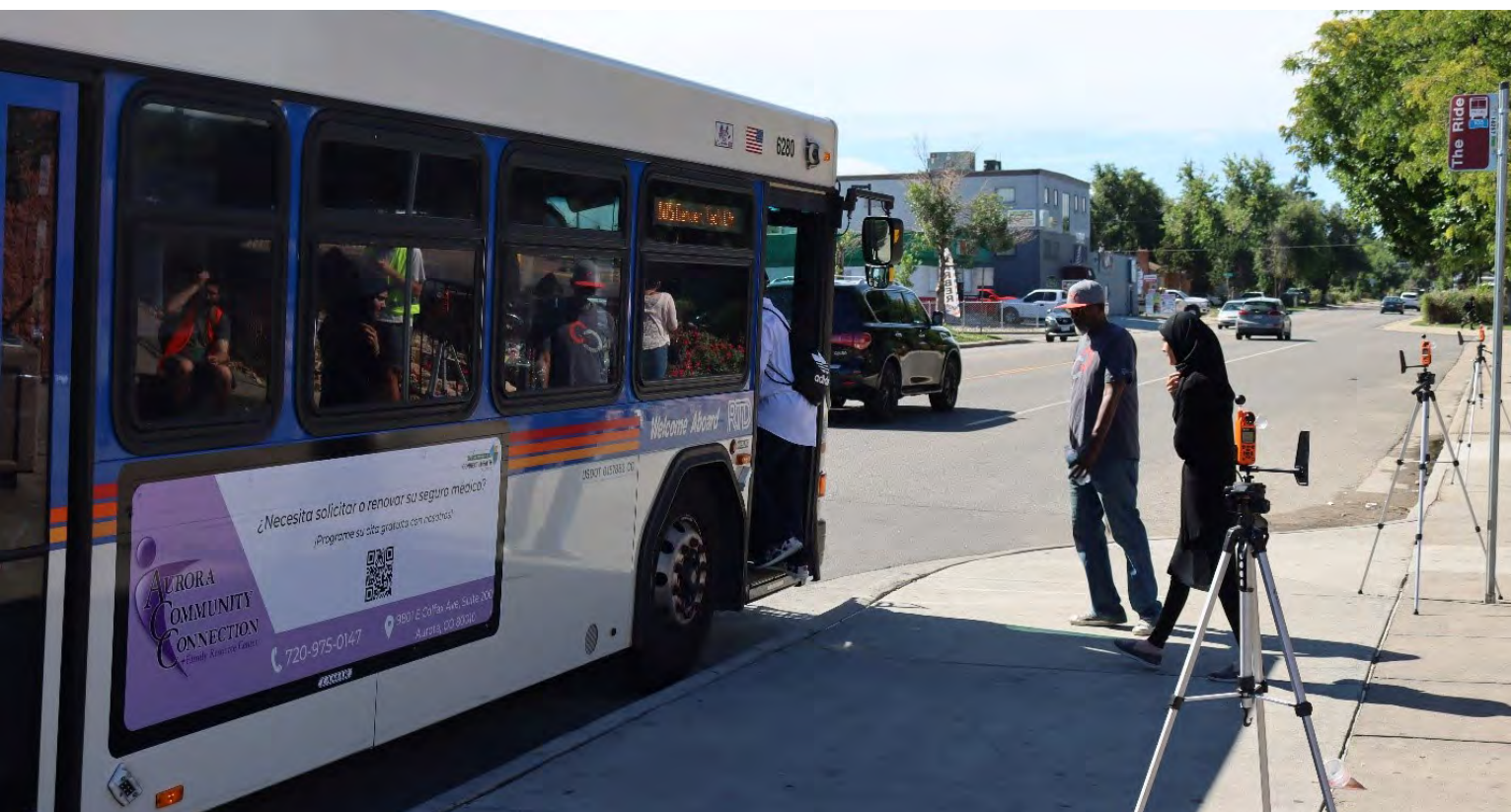
Researchers affiliated with the Denver Urban Field Station collected microclimate data at bus stops around Denver using portable weather stations called Kestrels. They also asked transit riders about thermal comfort during their commutes to understand if extreme heat affects some riders more than others—and how city managers could improve conditions. USDA Forest Service photo by Travis Warziniack
