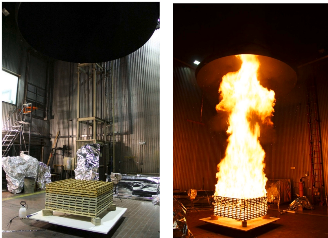
Fig. 1. Left: A photograph of the crib fire test prior to ignition. Right: An image of the steady burning achieved during the second test, showing the flame reaching up into the ventilation hood 6 m above.
