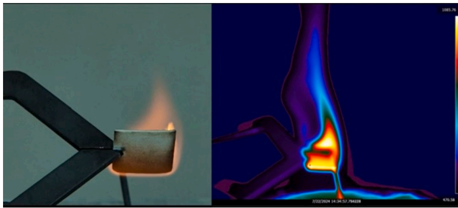
Fig. 5. Experimental measurement of ignition of inclined cellulosic leaf in 1048 K, captured by HD and IR camera.
