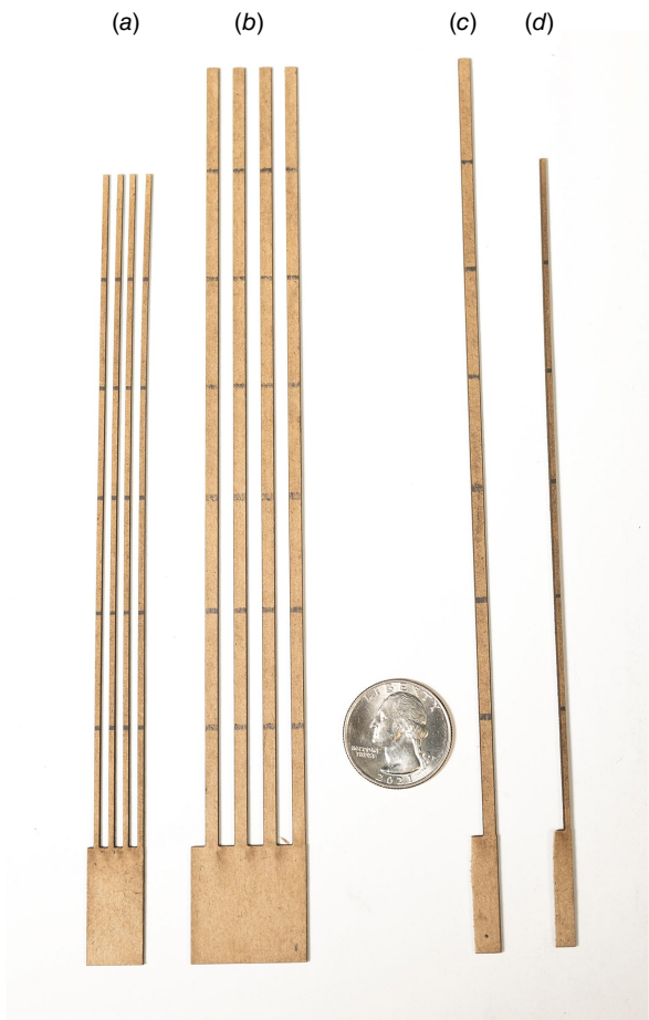
Fig. 2. Photograph of cardboard fuel elements used in experiments: (a) quadruple 1.578 mm wide, (b) quadruple 3.175 mm wide, (c) single 3.155 mm wide, and (d) single 1.578 mm wide.
