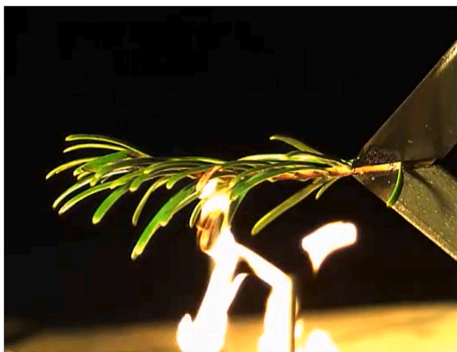
Fig. 5. Grand fir branch heated in 800 °C air. Image is a frame captured using a high-speed camera at 1000 fps showing flammable gases jetting from the needles, several seconds before the entire branch ignites.
