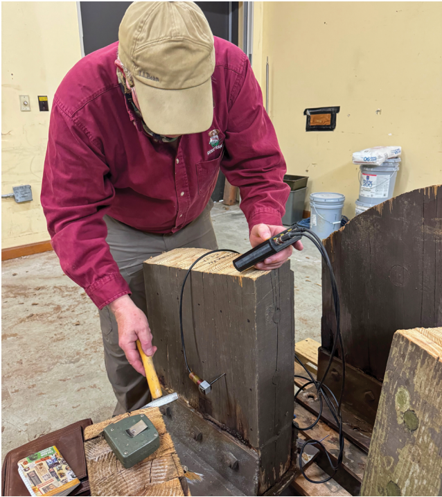
Figure 3. —Nondestructive testing of arch end sections (stubs). Courtesy photo by Laurice M. Spinelli Correa.
