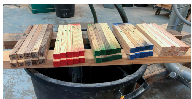
Figure 9. —Toughness specimens after processing, prior to moisture conditioning at 12 percent equilibrium moisture content. Courtesy photo by Laurice M. Spinelli Correa.
