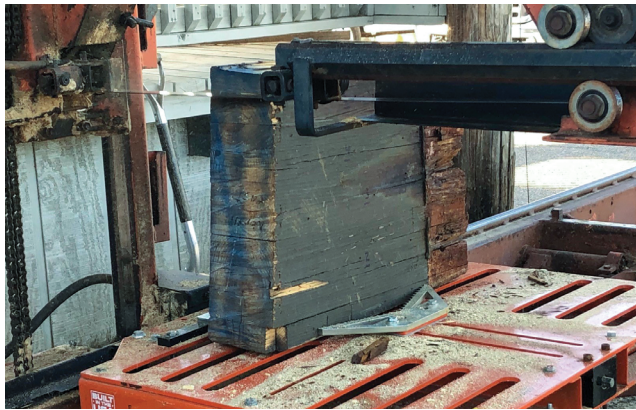
Figure 6. —Glulam stub on the bandsaw mill during lamina-of-interest recovery. Courtesy photo by Laurice M. Spinelli Correa.
