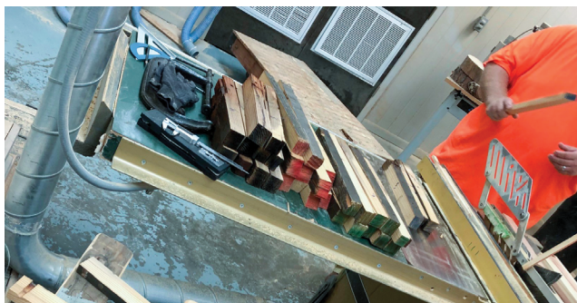
Figure 8. —Ripping operation by which 0.79 by 0.79 in. cross sectional toughness specimen blanks were recovered from each lamina of interest. Courtesy photo by Laurice M. Spinelli Correa.
