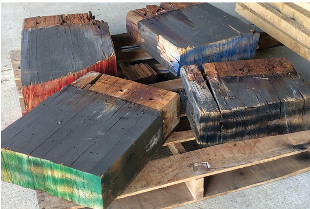
Figure 4. —Glulam stubs after steel anchorage shoe removal and color coding. Courtesy photo by Laurice M. Spinelli Correa.
