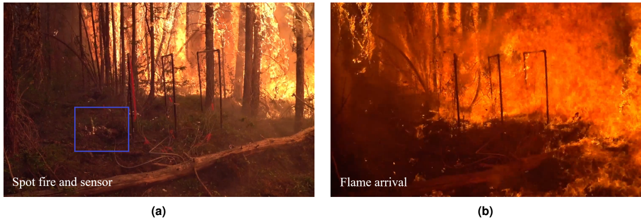
Figure 3. Still images from in-fire video (a) before the arrival of the fire front while a spot fire ignited near the sensor, and (b) as the flame front initially arrives. The blue box in (a) contains both the spot fire and sensor. The camera is pointed approximately east. Photo Credit: Greg Baxter, FPIInnovations
