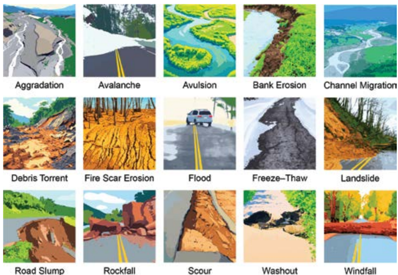
Figure 4.1—Ways that the effects of climate stressors, climate change, and other disturbances affect roads and other infrastructure. Multiple pathways are common. Figure from Strauch et al. (2014).
