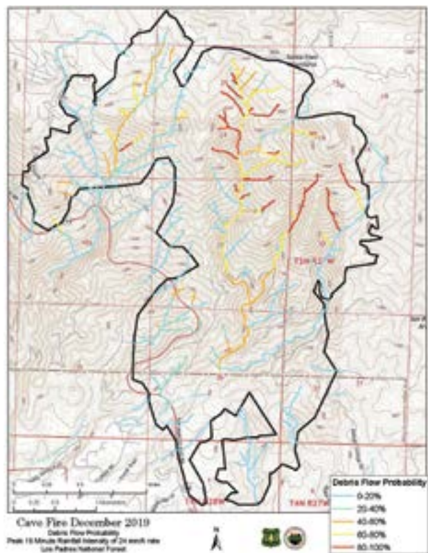
Figure 4.16—Example of a U.S. Geological Survey debris-flow hazard map with debris-flow probabilities for the 2019 Cave Fire, Los Padres National Forest.
