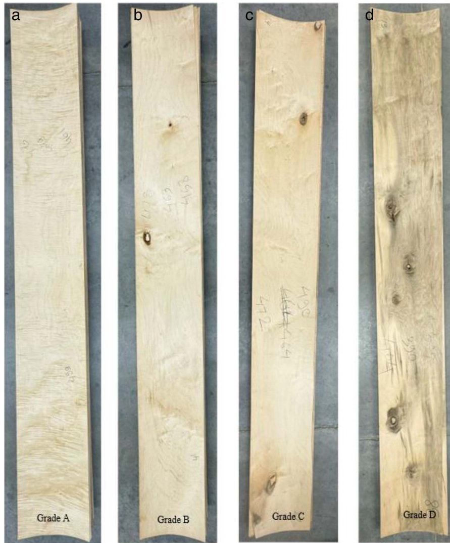
Figure 1.—Visually graded veneer specimens: (a) Grade A, (b) Grade B, (c) Grade C, and (d) Grade D.
