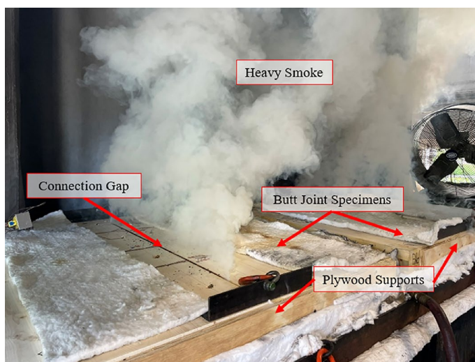
Fig. 6 Butt joint connections during testing
