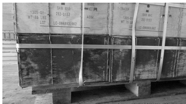
Figure 1. Wire-bound boxes on shipping pallet with substantial mold growth.
