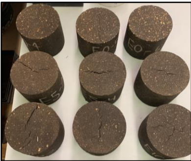
Figure 4. Visual Damage to Sand Asphalt During CP7 Conditioning
