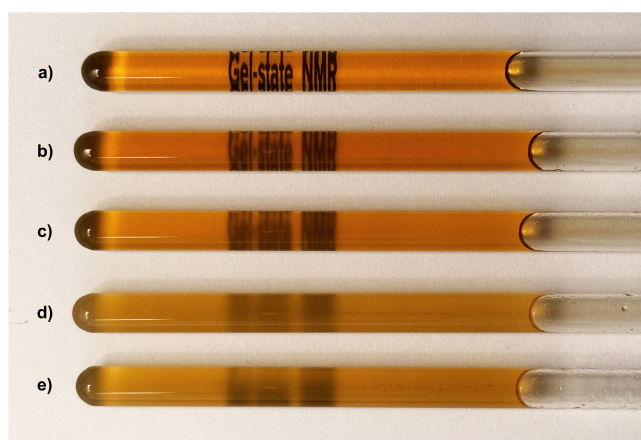
FIGURE 1 | Ball-milled aspen cell wall (CW) samples in NMR tubes from different preparation conditions (ball milling condition: 15 min grinding×11 and 8 min break; total grinding time: 4 h 5 min for 200 mg CW): (a) Freeze-dried CW in DMSO- d 6 /DMF- d 7 (4:1, v/v), (b) oven-dried (48 h) CW in DMSO- d 6 /DMF- d 7 (4:1, v/v), (c) oven-dried (16 h) CW in DMSO- d 6 /DMF- d 7 (4:1, v/v), (d) air-dried CW in DMSO- d 6 /DMF- d 7 (4:1, v/v), and (e) air-dried CW in DMSO- d 6 .
