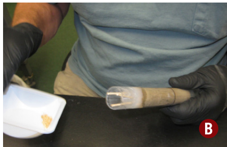
▲ Fig. 3. A Counted termites ready to be placed in tubes. B Termites placed into tubes. C Tubes during experiment.
