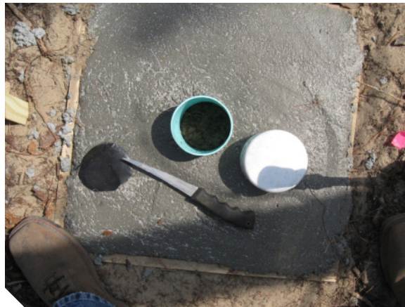
▲ Fig. 2. A day after treatment and concrete pouring, vapor barriers from within the PVC pipes are cut and removed. A wooden block is placed directly onto the treated soil, and the pipe is capped.
