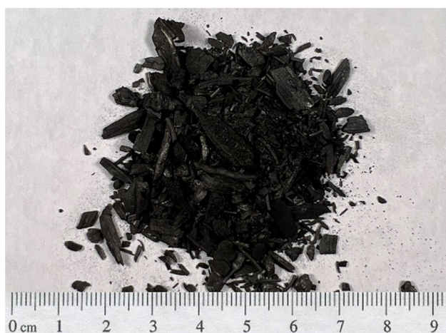
Fig. 1 Particles of the biochar used in the present study after separating from ash. (Biochar source: a local biomass combined heat and power plant in the central area of Maine, USA)
