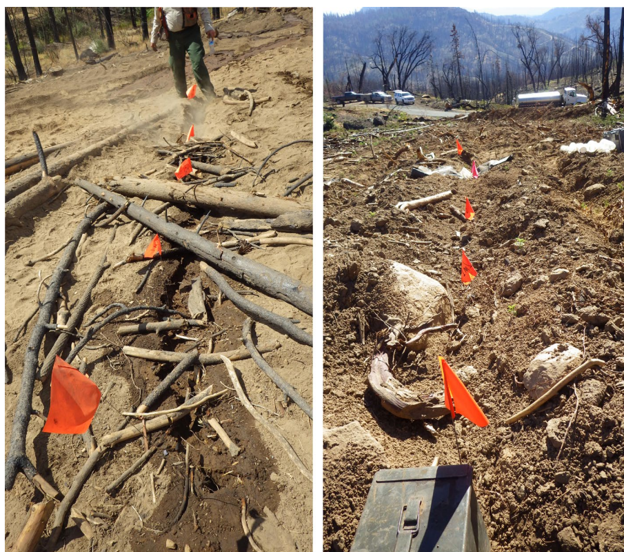
FIGURE 4 | The left panel shows the drop and lop treatment on a few pass skid trail after the rill experiment was completed. The wetted area is where the flow travelled down the skid trail and demonstrates the potential for incision that allows rills to pass under slash on the ground surface. The right panel shows the subsoiled treatment on a many pass low slope skid trail prior to the rill experiment. For reference, the flags are 1-m apart.
