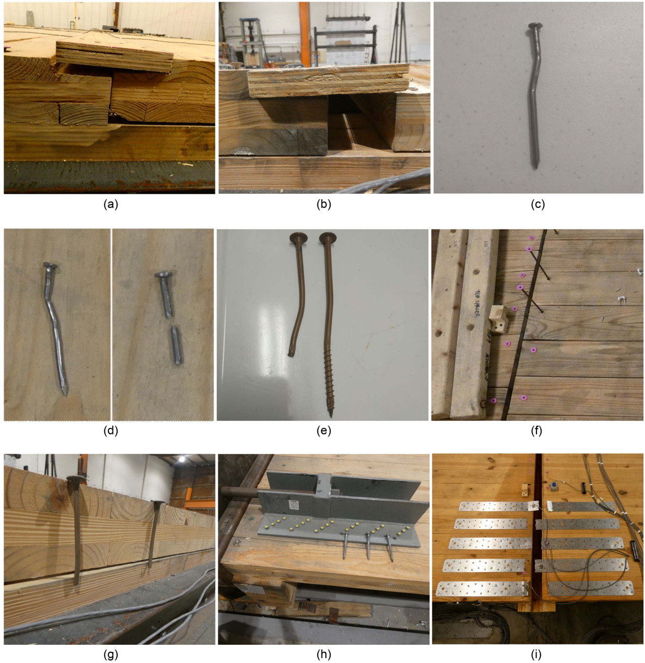
Fig. 15. (a) Spline deformation in first diaphragm test; (b) spline deformation in second diaphragm test; (c) nail deformation in first diaphragm test; (d) nail deformation in second diaphragm test; (e) typical CLT-glulam screw deformation for both diaphragm tests; (f) intact screws along Grid 2-2 for first diaphragm test; (g) screws along Grid 3-3 for second diaphragm test hung outside CLT for reference; (h) typical intact hold-down and screws after first and second diaphragm tests; and (i) tension straps rupture in first diaphragm test.
