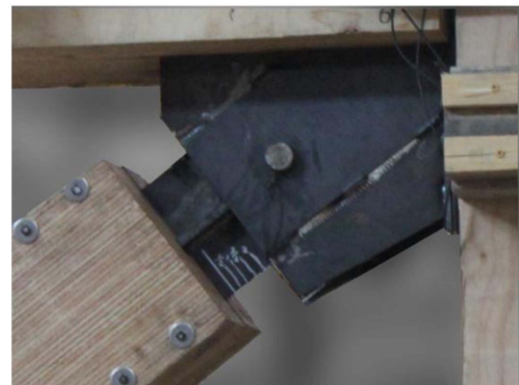
Fig. 7. Extension of TBRB core during Test TBRB1.
