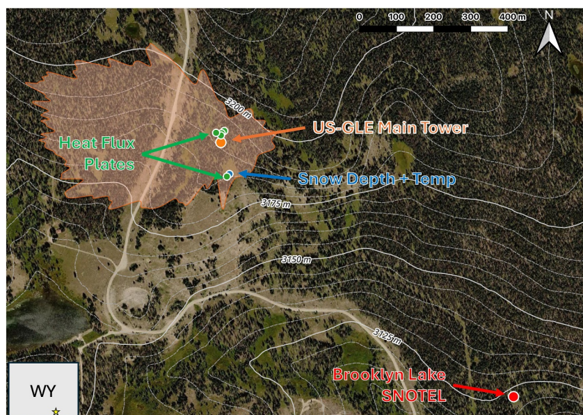
Figure 1. Map of the region around the US-GLE Ameriflux site. The points indicate the locations of the various sensor installations. Orange: main micrometeorology tower, green: soil heat flux plates, blue: snow depth and temperature probes, red: Brooklyn Lake SNOTEL site. The Orange polygon gives the 90% flux footprint for eddy covariance data at US-GLE. 5 m contour intervals are shown as white lines. The location of the site within the U.S. state of Wyoming is shown in an inset on the bottom left.
