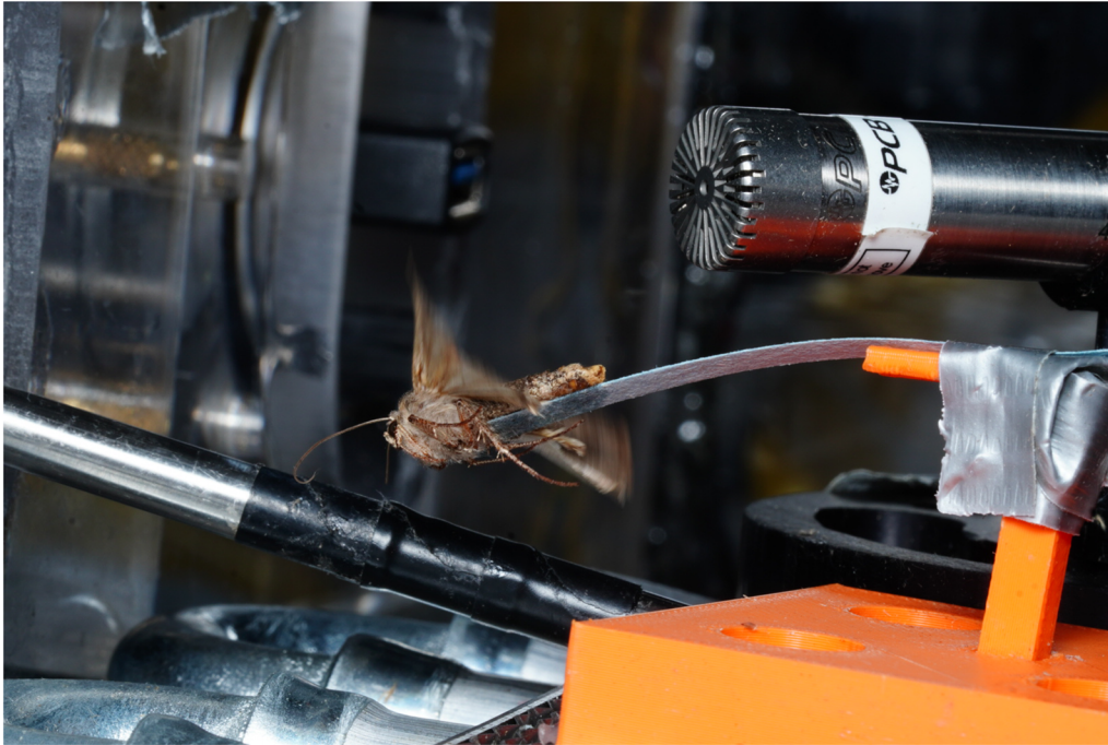
Fig. 2. Euxoa auxiliaris moth flying above a wall-mounted toggle, held stationary by a strip of paper affixed to the abdomen and taped to a 3D-printed stand. To the right of the moth is the piezoelectric microphone for wingbeat frequency recordings. Photo: T.E. Kennedy.
