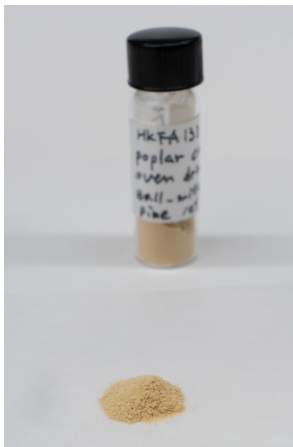
Lignocellulosic biomass from poplar that has been dried in an oven at 50°C and ground in a ball mill in preparation for analysis with gel-state 2D NMR. Forest Service photo by Nathaniel Sapp.
