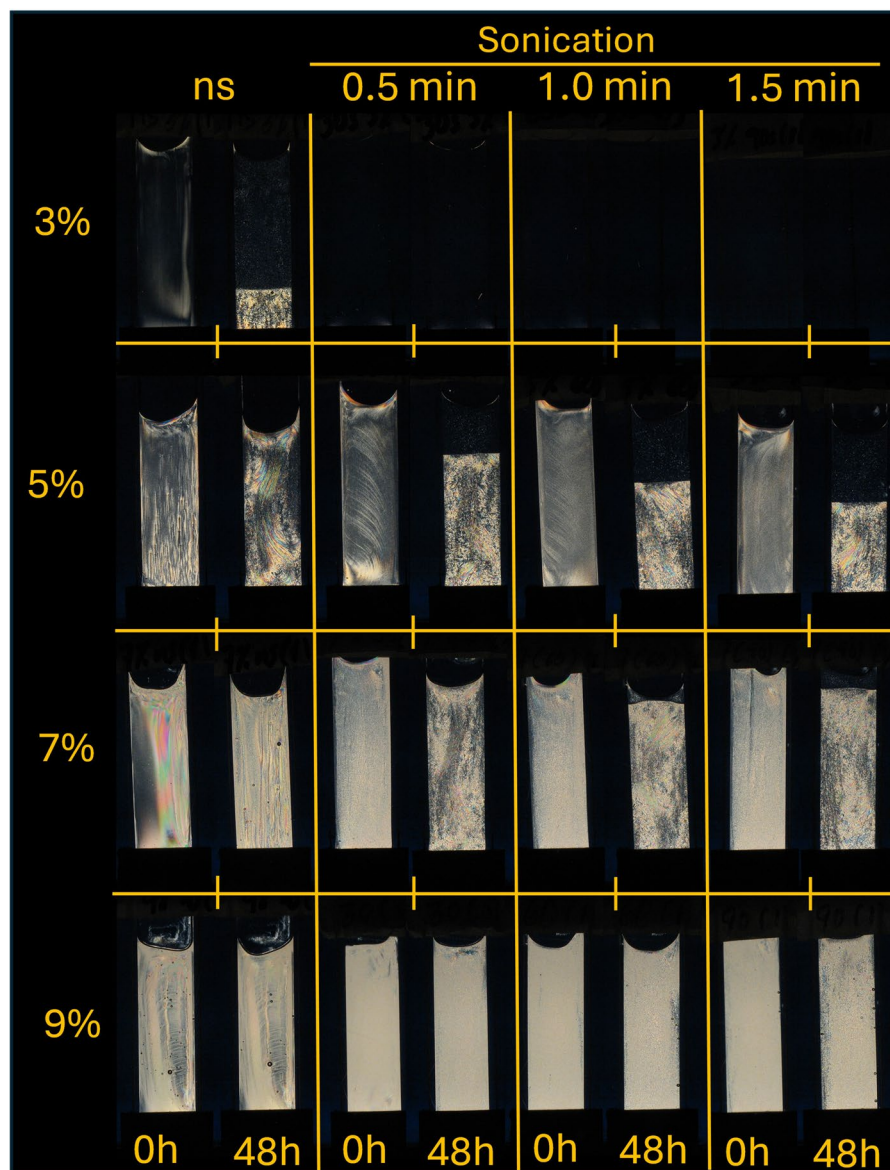
Fig. 2 CNC suspensions at different concentrations (3, 5, 7, and 9%) observed through crossed polarizers at 0 and 48 h. Brightness increased with higher concentration due to stronger particle interactions and alignment, reflecting higher birefringence. Over 48 h, structural reorganizations were observed, with brightness decreasing or shifting, indicating dynamic rearrangements in the CNC organization over time
