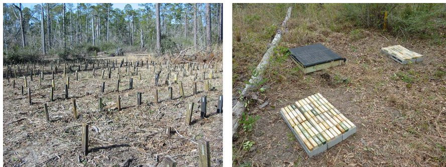
Figure 1.—Field exposure of test specimens in ground contact (left) and ground proximity (right) tests (photo credits: Stan Lebow and Rachel Arango).
