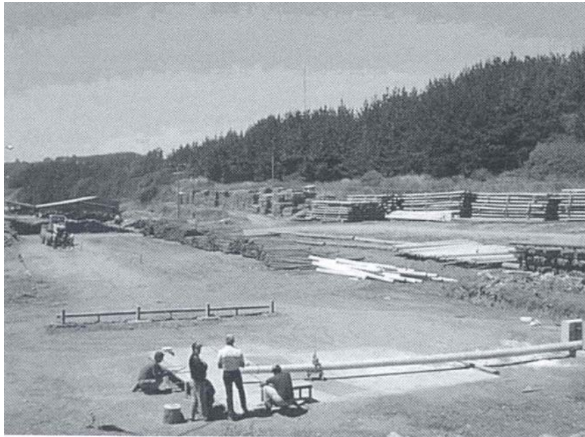
Figure 2.—Cable load placed 0.6 m from the tip is bending the pole as a cantilever beam.
