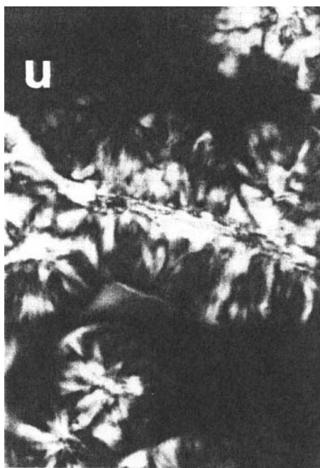
Figure 1 Fibers showing transcrystallinity in uncoupled kenaf-PP composites.
