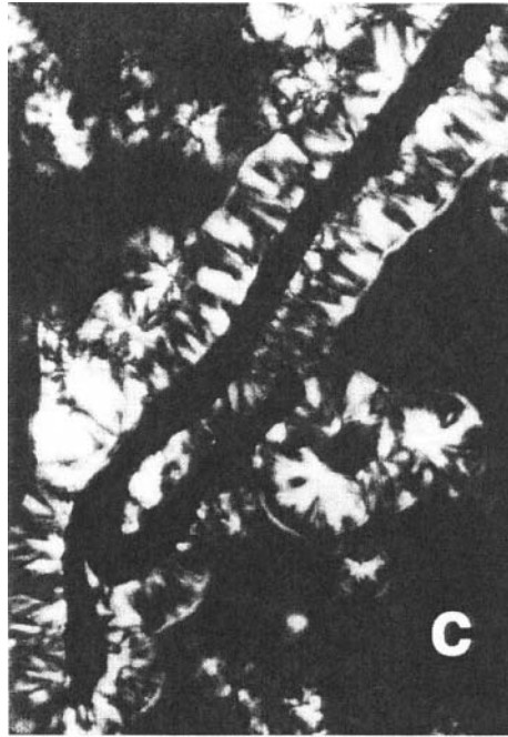
Figure 2. Fibers showing transcrystallinity in coupled kenaf-PP composites, with MAPP as the coupling agent.
