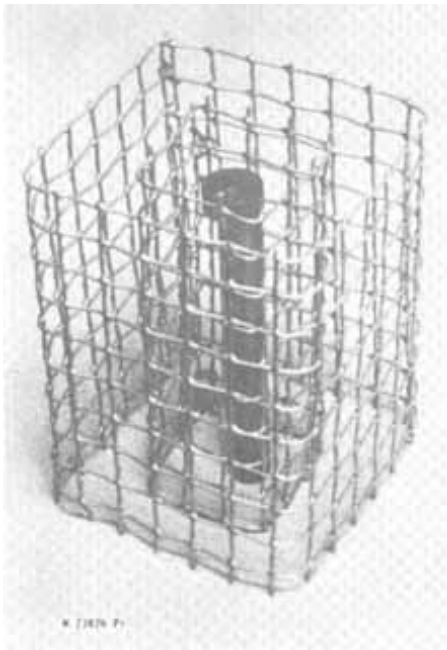
Figure B-1.—Apparatus for supporting test specimen and alcohol cup. Specimen to be supported on top wire strand. (M 77876 F)
