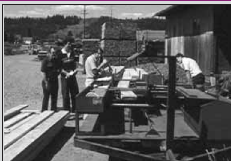
In-grade testing using portable equipment, 1980.
