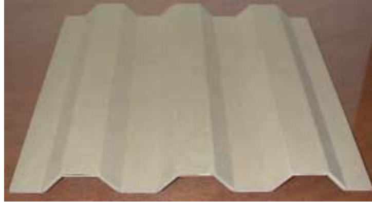
Figure 3 Preliminary design of a uniaxial corrugated core made from fiberized fibers from small diameter tree tops.
