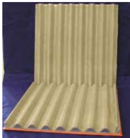
Figure 8 Aluminum mold designed to form 3D engineered fiberboard cores. Outside dimensions are 61 by 61 cm (24 by 24 inches).
