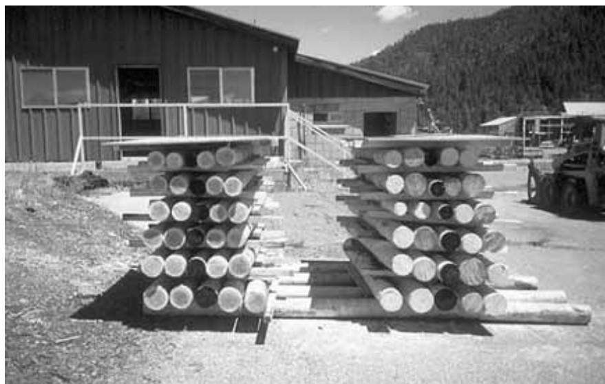
Figure 1. — Air-drying stacks of ponderosa pine and Douglas-fir logs in Hayfork, CA. Dark end-coated logs are logs used to monitor MC.
