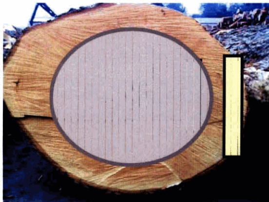
Figure 1. Log end showing the wood zone where wood quality and strength properties are diminished due to cellular changes and proximity to the pith (the two rectangles represent board locations). A board whose grain has less curvature is less likely to warp than a board with greater grain curvature.
